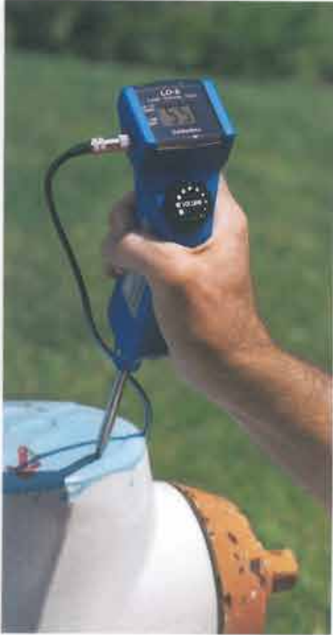
Listening at a Hydrant with a 4-inch Rod
