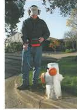
Which hydrant, valve or meter is loudest? Leak is closest to the loudest.
