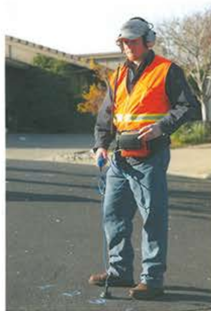
Listening at different spots to detect differences in loudness of the leak
