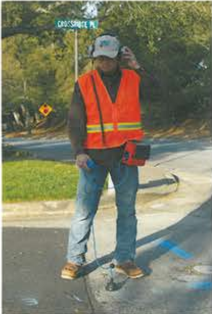
Listening with the LD-18 directly over the pipe
