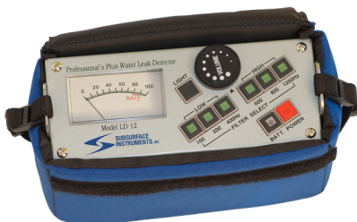
AMPLIFIER WITH METER DISPLAY AND FILTER CONTROLS
