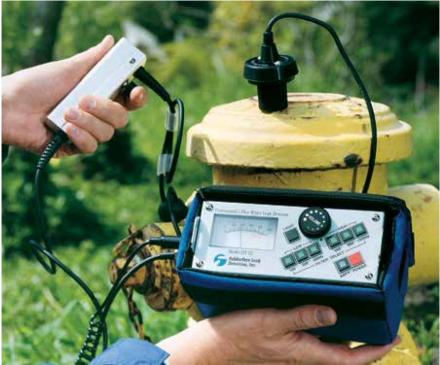
Figure 4-6 Leak Survey at a Hydrant
